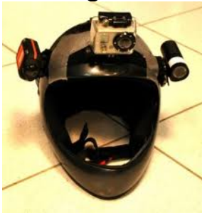
Four types of helmet mounted SD cameras Showing their positioning and small size.
